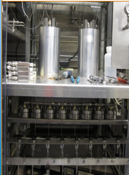
~1.4 cc 8-reactor packed bed system
