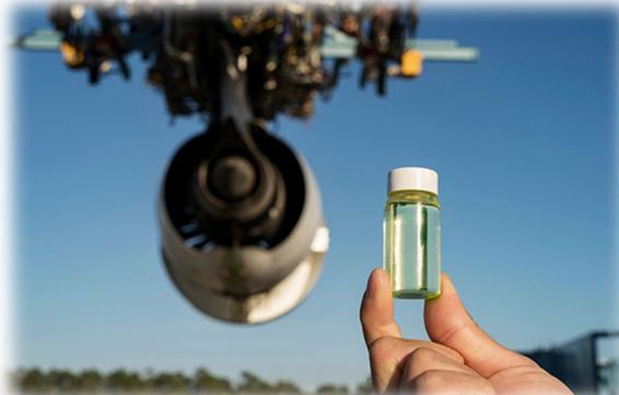
Pratt & Whitney PW1100G Advantage engine test – 100% HEFA-SPK.
