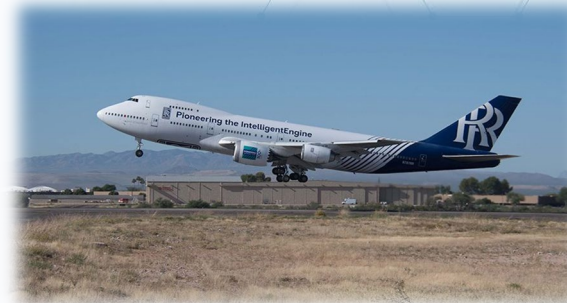
Rolls-Royce Trent 1000 engine flight – 100% HEFA-SPK.
