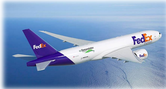
Boeing 777 EcoDemonstrator flight with GE90 engines. On-wing engine tests – 100% HEFA-SPK.
