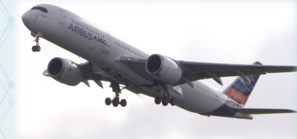
Airbus A350 Flightlab flights with Rolls-Royce Trent engines – 100% HEFA-SPK.
