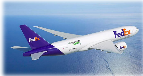
Boeing 777 EcoDemonstrator flight with GE90 engines. On-wing engine tests – 100% HEFA-SPK.
