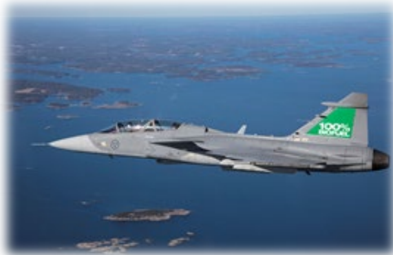
Swedish MoD Gripen flight with GKN RM12 engine (GE F404 derivative) – 100% CHJ.
