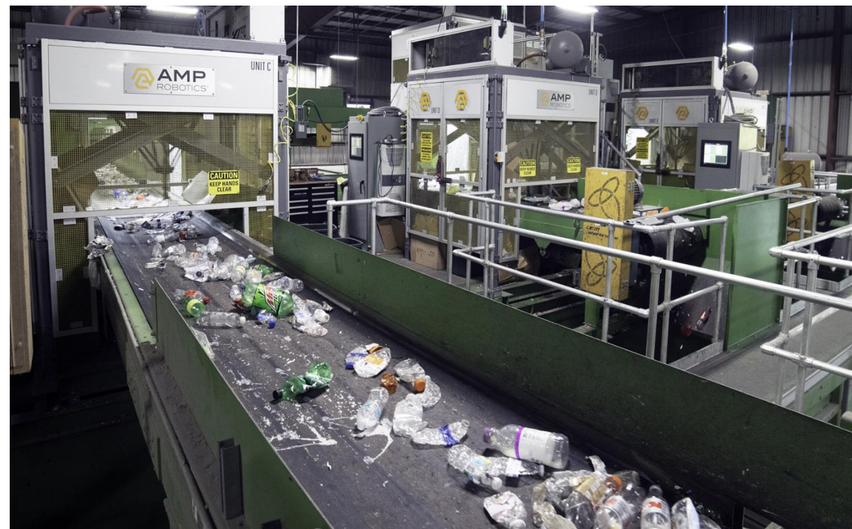
AMP's AI computer vision systems and robots operating in a single- stream recycling facility
